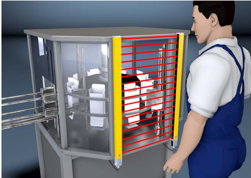
Figure 5.1: Point of operation guarding protects reaching into the danger zone, e.g. for cartoners or filling systems
